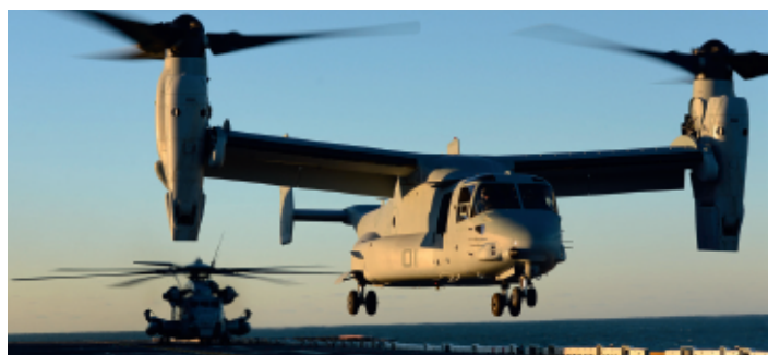
VARS-equipped Osprey will provide ship-based refuelling capability
