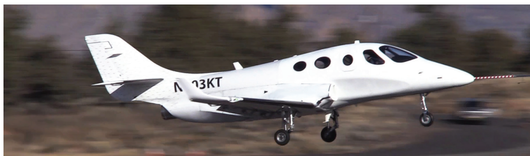
Single-engined type has a projected range of 1,500nm and Mach 0.7 top speed with four passengers
